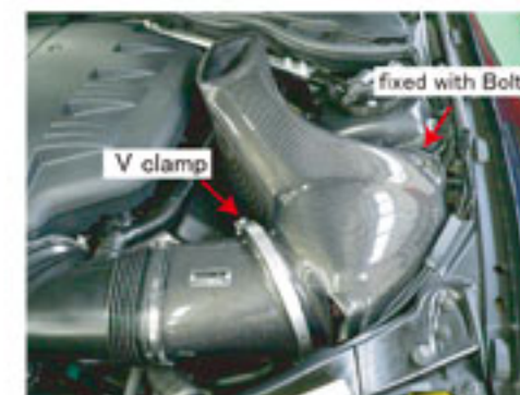
A filter is packed into the filter case A and it fixes by V clamp. It arranges so that a cleaner case may turn with a bottom down completely.
