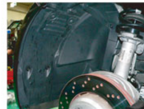
A bumper and an inner fender are returned, a tire is installed and cars are set down.
