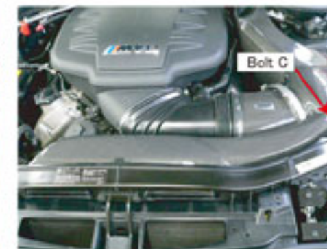
The carbon introduction duct B is installed and it fixes with Bolt C. The filter case A is fixed with Bolt B. V clamp is fastened and done simultaneously.
