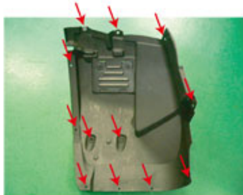
The air duct of an original bumper is removed. A left tire is removed and an inner fender is removed. (An arrow area is a fixed position of a bolt and a tapping screw)
