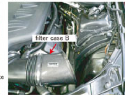
The filter case B is installed in a suction hose.
