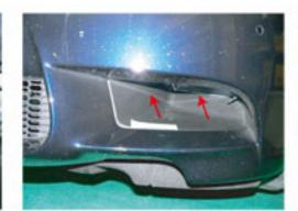
The tapping screw which is fixing the air duct is removed.
