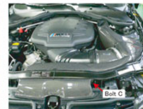
Double-stick tape is removed, the carbon introduction duct A is installed, and it fixes with Bolt C. Finally please confirm clearance with a bonnet.
