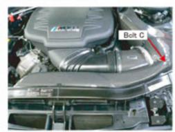
The carbon introduction duct B is installed and it fixes with Bolt C.
