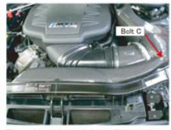
The filter case A is fixed with Bolt B. V clamp is fastened and done simultaneously.
