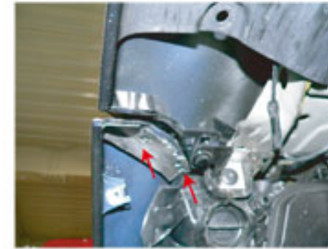
Because the tapping screw of the upper surface part is hidden by the bumper when removing an air duct, the bolt and tapping screw of an arrow area are removed and a bumper is freed.
