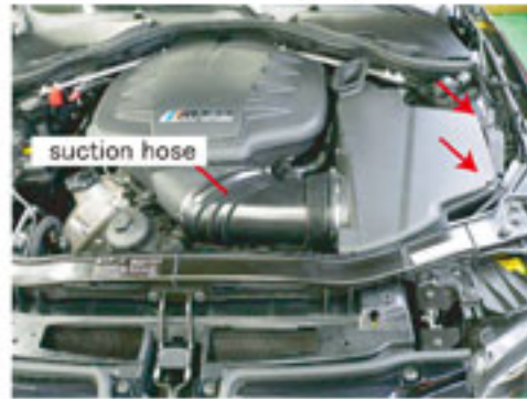
A blow by hose is left as it is, and removes a suction hose once first. The fixed bolt of an arrow area is removed and a filter case is removed.
