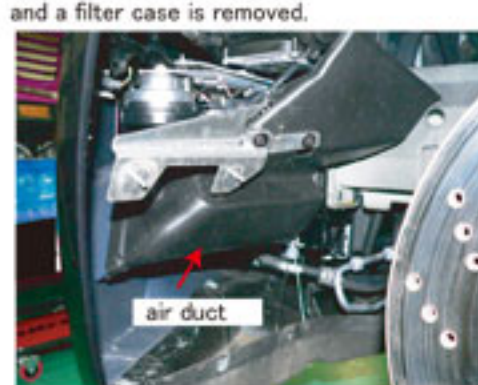
An inner fender is removed and then an air duct is removed.
